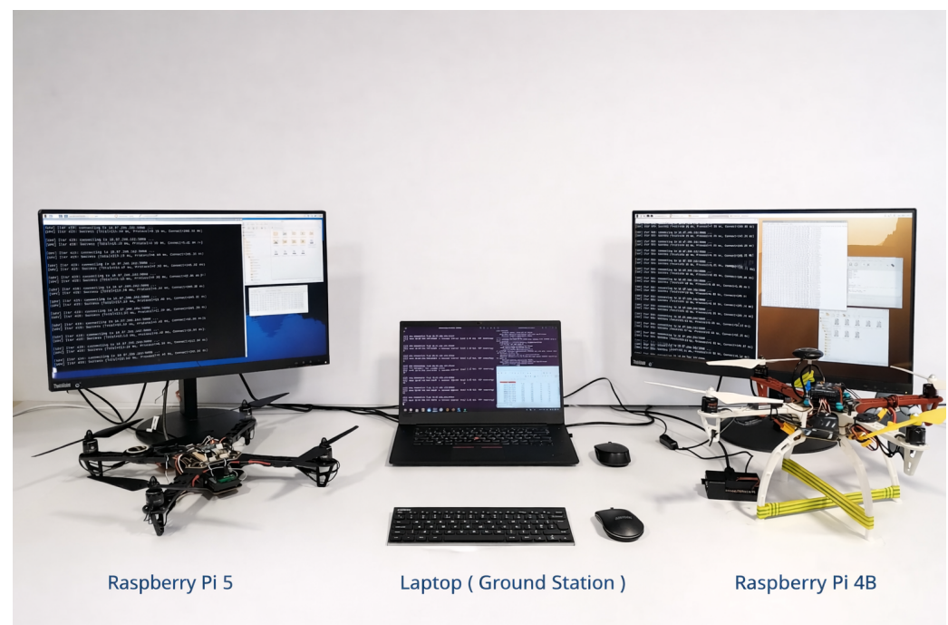
Figure 7. Experimental testbed used for latency evaluation. The ground station runs on a laptop, while the UAV node is implemented on Raspberry Pi 4B or Raspberry Pi 5 in separate experimental runs. All nodes communicate over IEEE 802.11.
