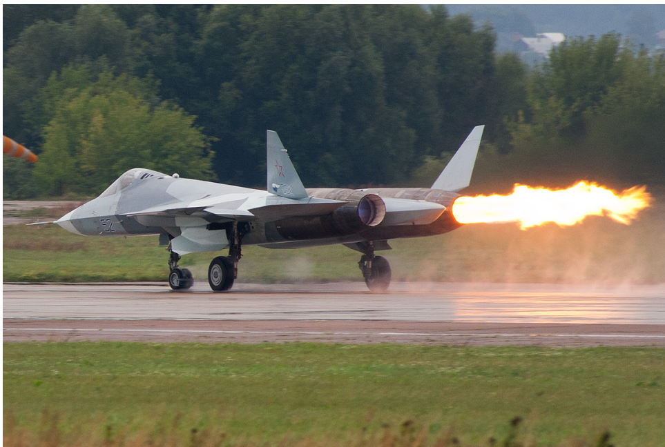
Fig. 1.1: Sukhoi Su-57 prototype suffering a compressor stall at MAKS 2011 [1].
