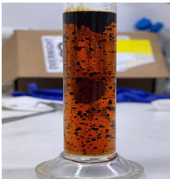
Figure 5-9 Biooil from test 6 containing high-water content with solubilizing acids, alcohols and ketones from carbohydrate decomposition [214]
