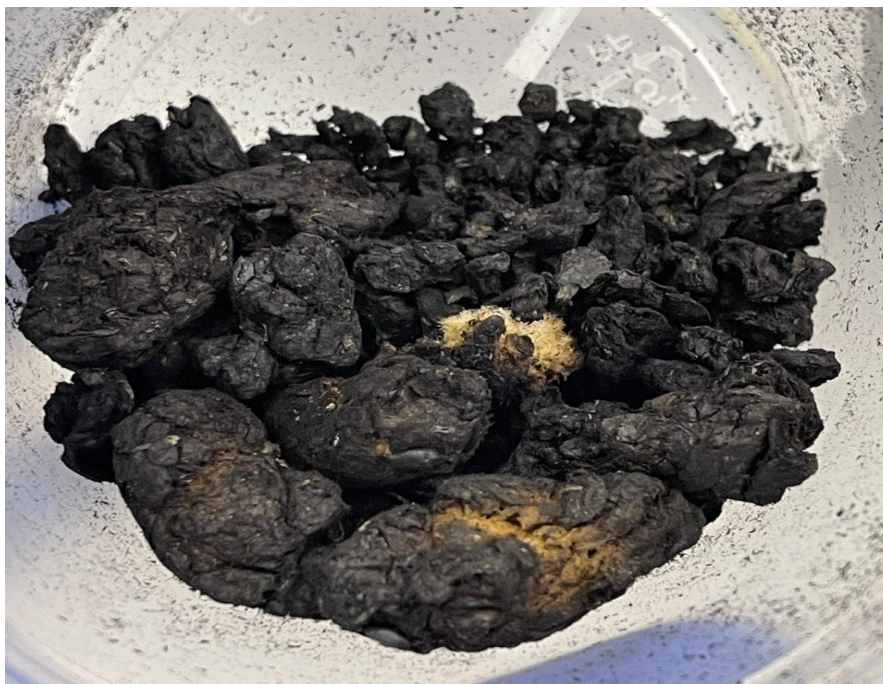
Figure 5-6 Incomplete conversion of char obtained from test 1 at 375°C
