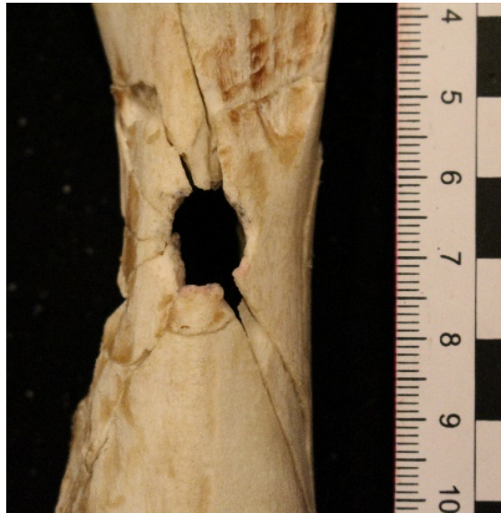
Fig 6 A porcine target impacted with a lead sphere
