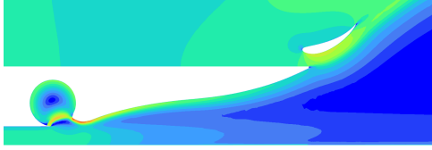
(c) TVC at airfoil-shaped diffuser, with mass-flow rate V_{in}/V_{\infty} = 2
