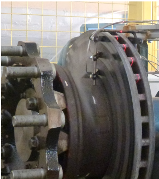
Figure 21: Smoke tests - evidence of exiting ID airflow causing the upper inlet blockage (laser red light marking rotor mid-plane)
