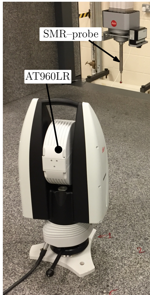
Figure 5.2: An AT960LR laser tracker fixed to the large granite base of a Leitz PMM-F 1000 CMM. The tracker is locked onto an SMR-probe that is moving to probe the surface of the CMM base. The tracker is measuring the position of the SMR in spherical coordinates.
