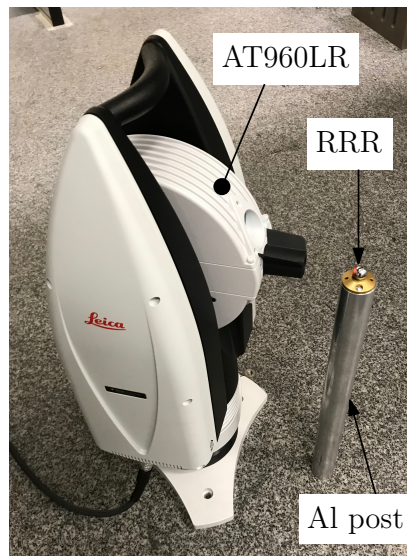
Figure 5.10: An AT960LR installed on the base of a CMM. The tracker interferometer is locked onto an RRR that is fixed in a three-point hold on an aluminium post. The post height is designed to hold the RRR close to the plane of the laser tracker’s equator. The distance between tracker home position and RRR was minimised.
