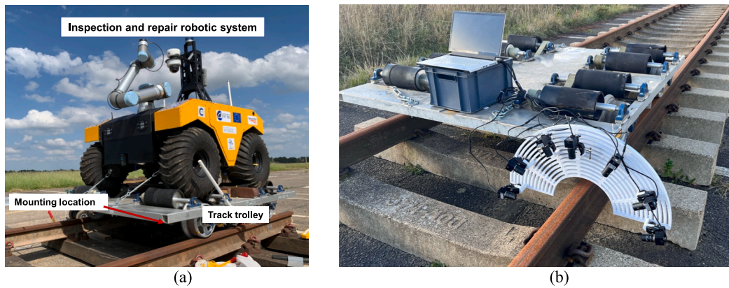
Fig. 12. (a) The robotic platform [43,44]. (b) System integration on the front base trolley.
