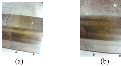
Fig. 8. Snapshots of different working distances at the angle of 60°. (a) working distance: 38 cm; (b) working distance: 30 cm.
