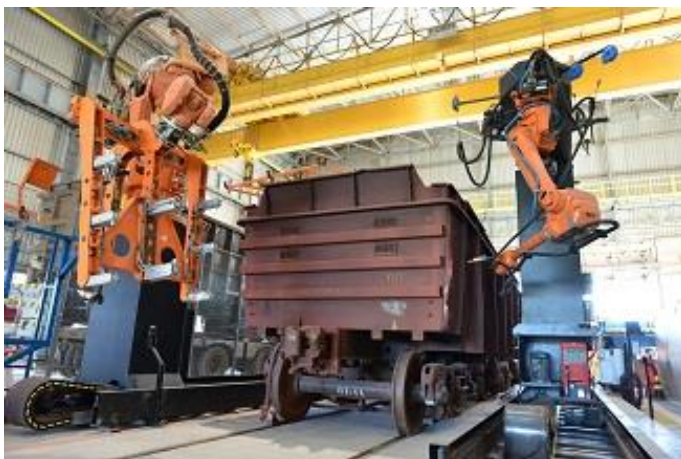
Figure 2.10 Robot used for repairing rail car in mining operation [116]
