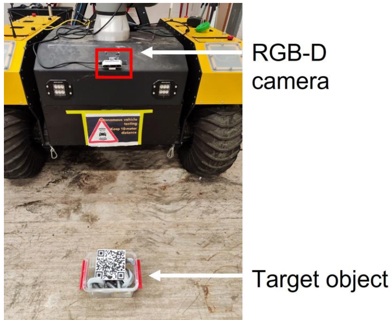
Figure 4.24 Automatic waypoint generation based on detected object
