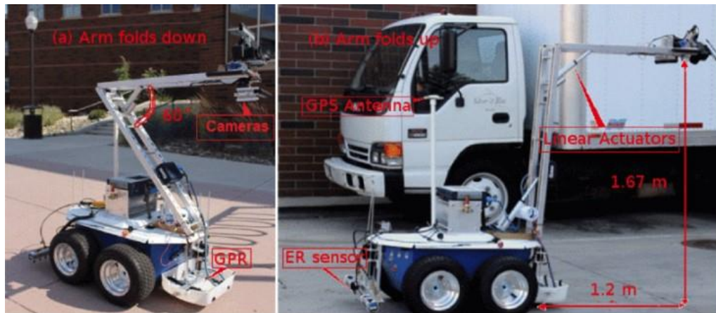
Figure 2.19 Proposed mobile manipulator system for with multiple sensors [150]
