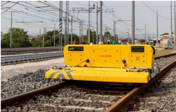
Figure 2.7 Felix in operation to inspect switch and crossing [91]
