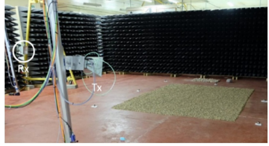
FIGURE 2 Image shows the Ground-Based Synthetic Aperture Radar (GBSAR) system in a bistatic configuration, with a gravel rectangle as the scene.
