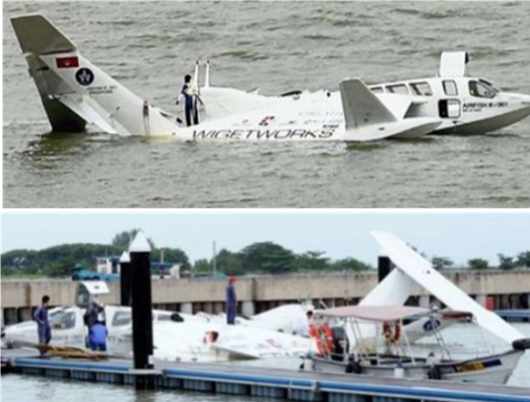
Figure 1-11 Photos of the damaged WigetWorks vessel, at sea awaiting tow (upper) and once returned to the quayside (lower). Note the extreme angle of the horizontal stabiliser indicating structural failure of the tail section
