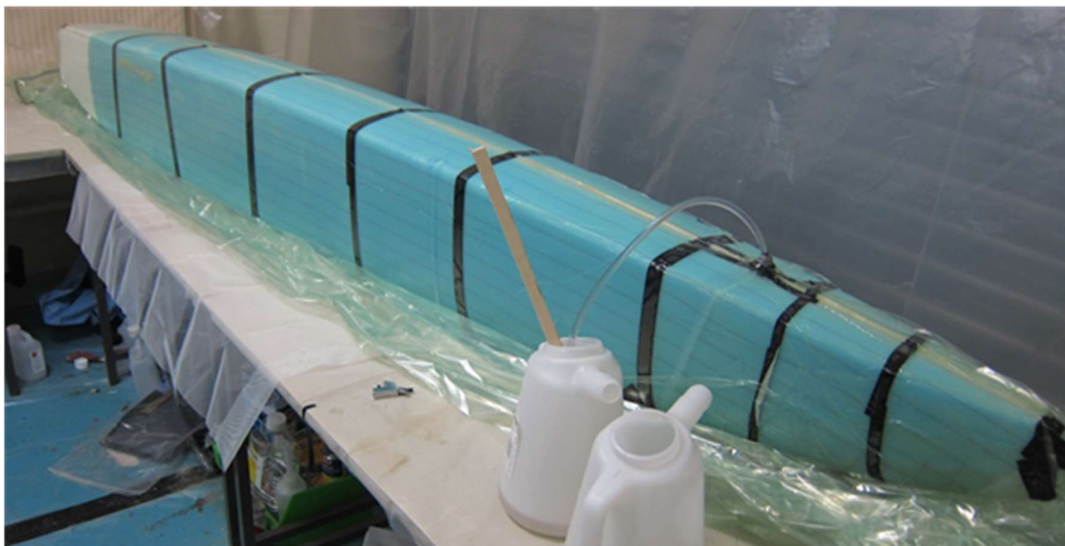
Figure 2-5 Process of the model lamination: from top, bare foam plug, inverted and wrapped in glass fibre, then vacuum bagged during the resin infusion process. The line of advancing resin can be seen toward the stern
