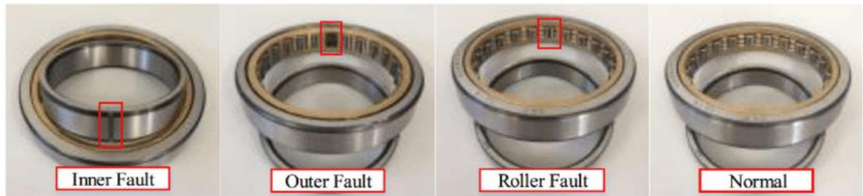
Fig. 1 Faults in the inter-shaft bearing [21].
