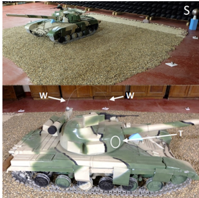
Figure 5-5: Photographs of model tank target. The wire on top is denoted by "W", the turret of tank denoted by "T", and the reference sphere is denoted by "S".
