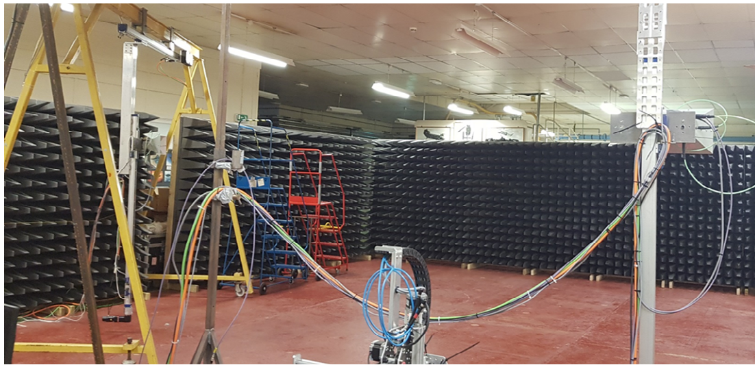
Figure 2-13: Experimental set up of Cranfield GBSAR laboratory. The antennas shown here are in the bistatic/multistatic configuration [136].
