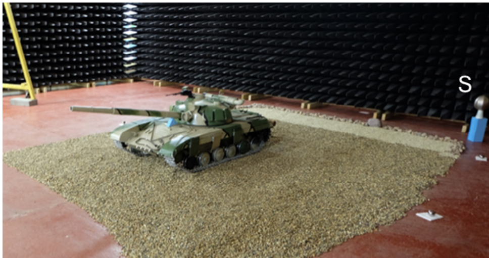
Figure 4-4: Target scene, consisting of a Quarter scale T72 tank model on gravel and reference sphere “S”.
