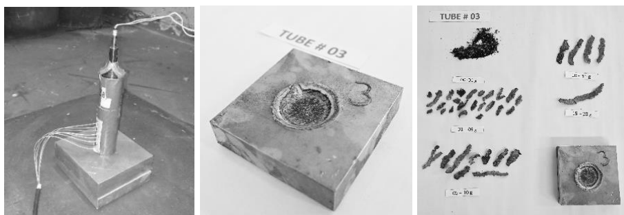
Figure 1.1: Experimental setup (left), witness plate indentation (middle) and fragmentation pattern (right).
