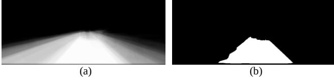
Fig 2. (a) road probability, the darker the pixel color the lower the probability the pixel belongs to the road (b) corresponding training mask.
