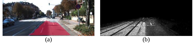
Fig 3. (a) example input image with outlined training mask (b) road segmentation obtained as P_r(u, v) \cdot P_{lr}(u, v) . (best seen in color)
