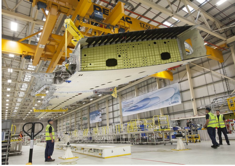
Figure 1.1: The process of wing assembly
