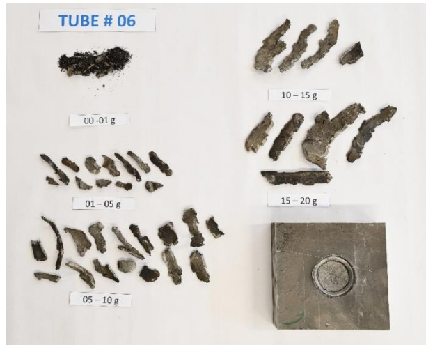
Figure 2-7: Small-scale detonation of UHP under heavy confinement.
