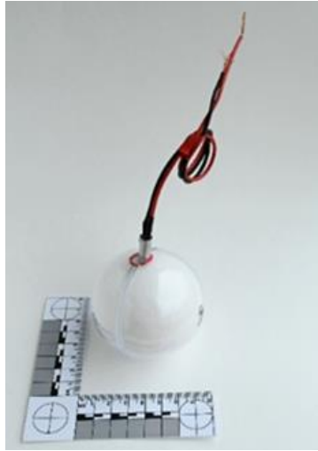
Figure 3-5: 100 g UHP charge configuration.
