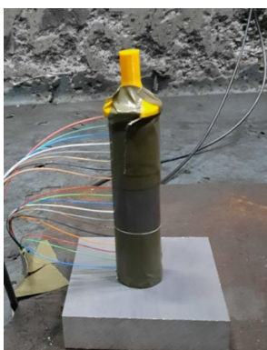
Figure 3. UHP (90 g) under heavy confinement – VoD stationarity assessment using 19 GOF.
