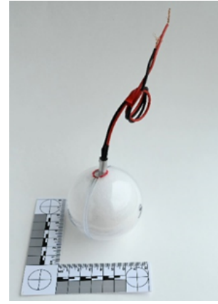
Figure 5. 100 g UHP charge configuration.
