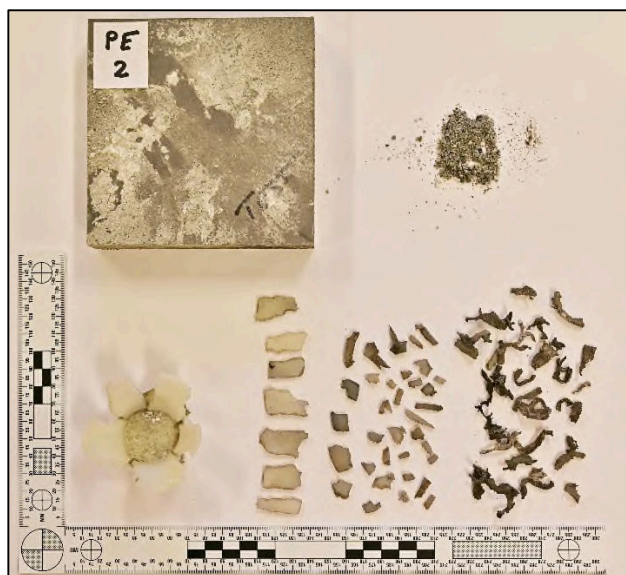
Figure 6. Light confinement – failed detonation: absence of indentation in the plate, presence of unreacted UHP and fragmentation pattern, including petalling of the bottom of the tube.
