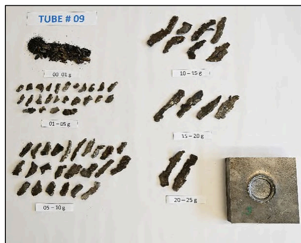
Figure 3. Fragmentation (90% mass recovery) and indent on witness plate for a confined 90 g UHP charge at density 0.83 g/cm 3 .
