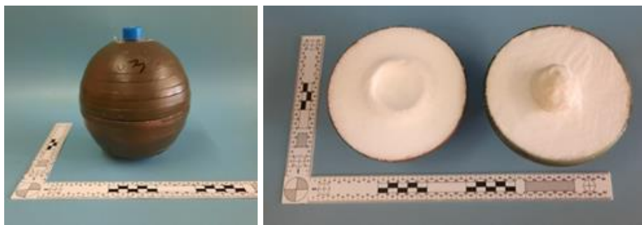
Figure 3-6: 1 kg UHP charge configuration.
