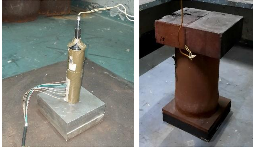
Figure 2-4: Setup for detonation of confined UHP charge with vertical initiation, witness plate, anvil, optical probes (left), protective structure to optimise fragment recovery (right).
