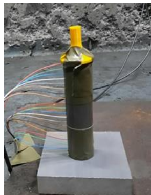
Figure 4-3: UHP (90 g) under heavy confinement – VoD stationarity assessment using 19 GOF.
