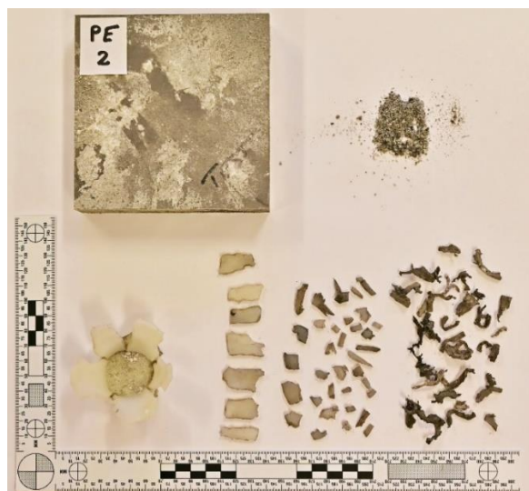
Figure 2-6: Light confinement – failed detonation: absence of indentation in the plate, presence of unreacted UHP and fragmentation pattern, including petalling of the bottom of the tube.
