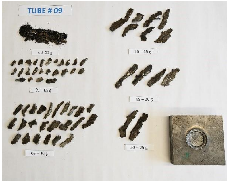
Figure 2-3: Fragmentation (90% mass recovery) and indent on witness plate for a confined 90 g UHP charge at density 0.83 \text{ g/cm}^3 .
