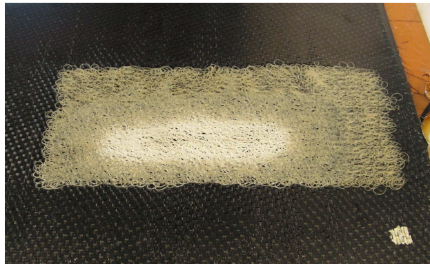
Figure 5.7: Dry spot within a densely tufted area of a cured panel
