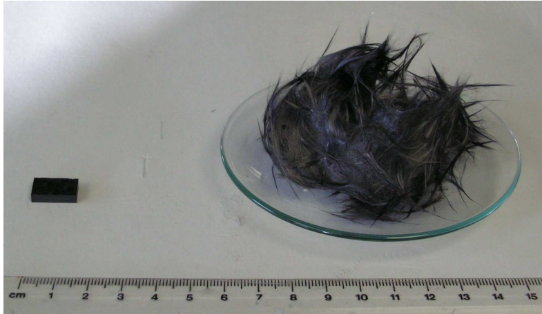
Figure 8.5: On the left composite sample before digestion, on the right dry fibrous residues of a sample of equivalent size.
