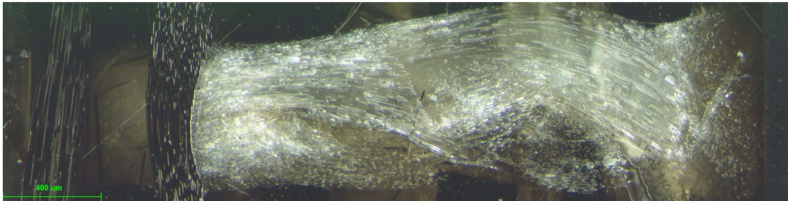
Figure 7.11: Dark-field micrograph of polished cross-section of cured glass fibre tuft. The ‘threaded’ shape of the tuft due the highly twisted yarns is visible.
