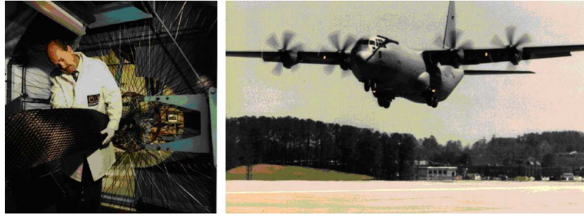
Figure 2.5: Left: 2D Braiding process for blade manufacturing. Right: Lockheed Hercules C-130J with composite blades, courtesy of R. J. McCarthy, Dowty Propellers (England).
