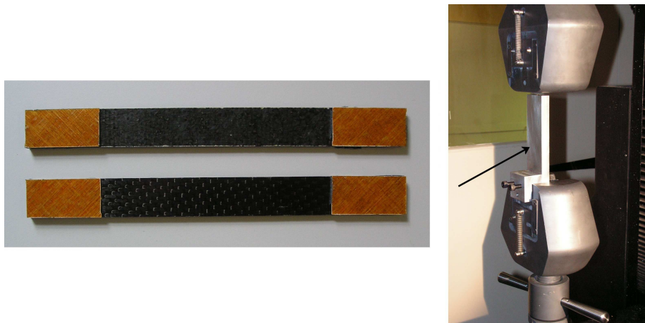
Figure 4.16: Left: tensile coupons with glass fibre tabs, tufted (top) and unreinforced control (bottom). Right: detail of specimen aligning guide for tensile testing fitted on Instron jaws (black arrow).
