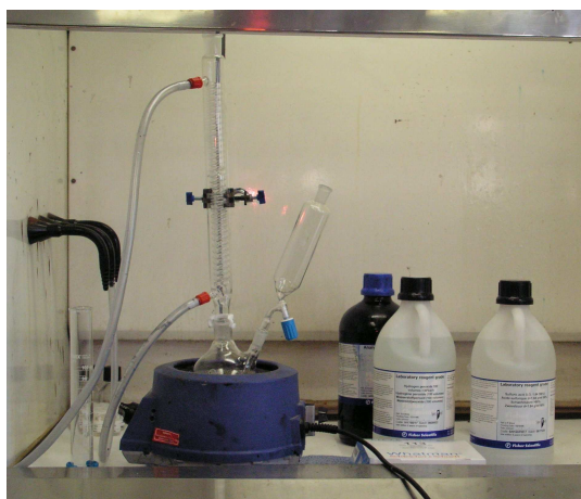
Figure 8.4: 'Digesting' unit for removing resin from composite samples
