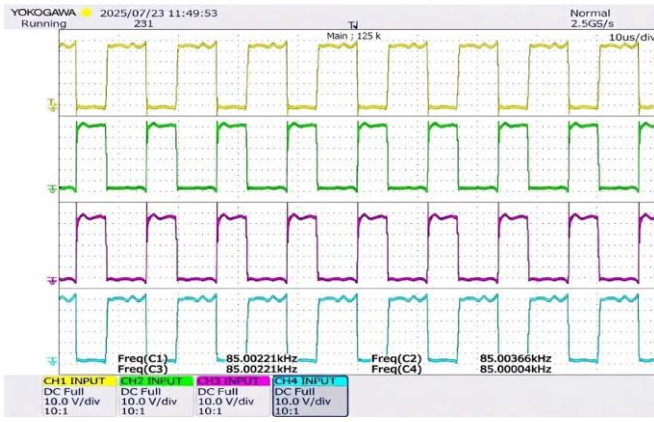
Fig. 10. Measured voltage waveforms across each inverter switch in the experimental square-wave WPT setup.
