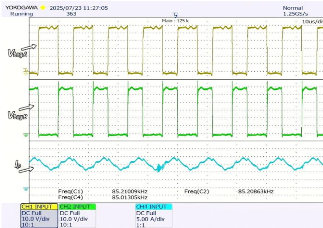
Fig. 11. Experimental waveforms of the LLM generated WPT system: inverter leg switching voltages and primary coil current at an operating frequency of 85.2 kHz s(60 V input, 10 Ω load).
