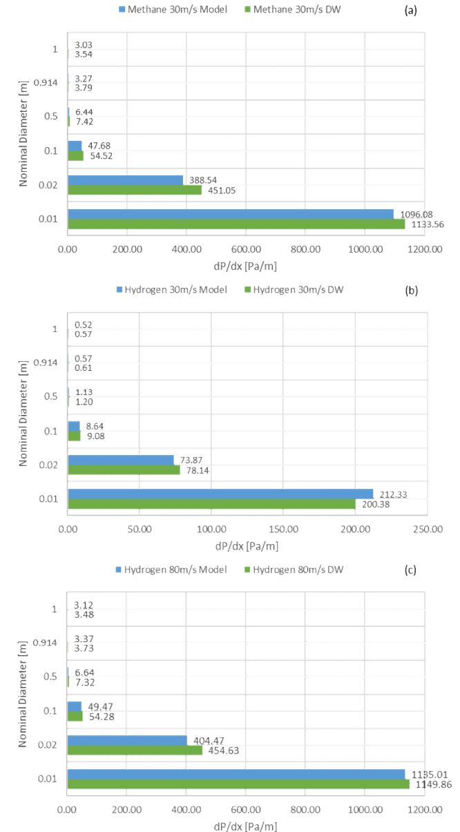
Fig 4. Comparing mathematical model (DW equation) to computational model (k-e model) based on pressure losses observed for (a) Methane with velocity 30m/s; (b) Hydrogen with velocity 30m/s; and (c) Hydrogen with velocity 80m/s in a steel pipe
