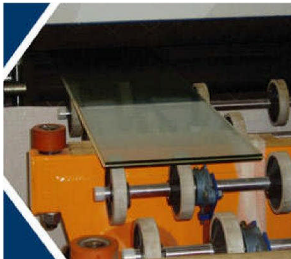
Figure 5. Heated roller system to soften interlayer and remove air bubbles. (Independent Glass Co Ltd, 2009).
