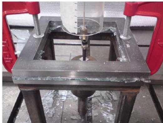
Figure 25. Original test setup post failure of single ply annealed float glass.
