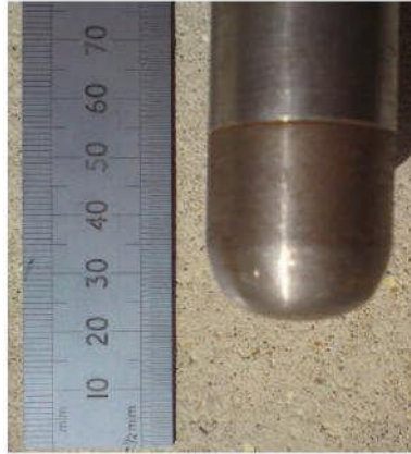
Figure 14. Original test impactor with reference scale.
