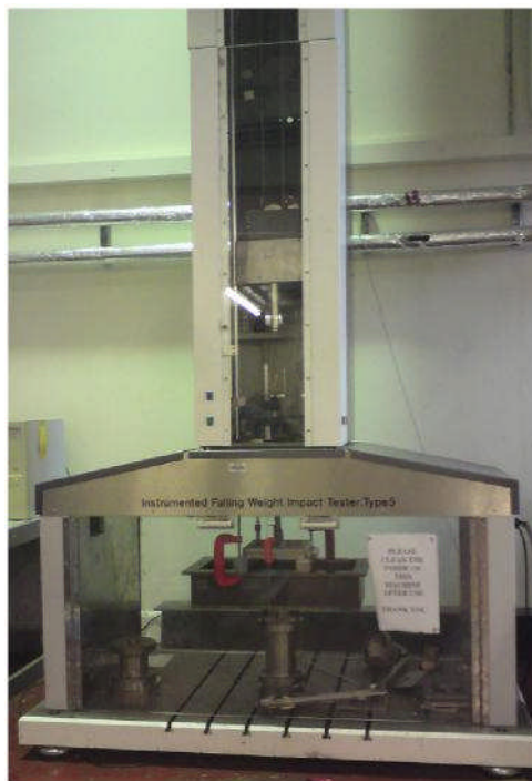
Figure 26. Type 5 Rosand Instrumented Falling Weight Impact Tester.
