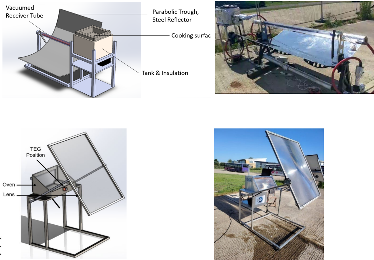
Figure 1. a. CAD model and built version of the PTC Cooker b. CAD and built version of the Fresnel cooker.
