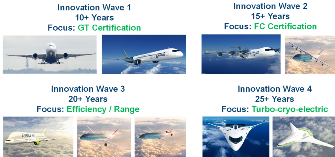
Fig. 2. Liquid hydrogen-fuelled aircraft innovation waves for gas turbine (GT) and fuel cell (FC) power (Images sources [6,16]).
