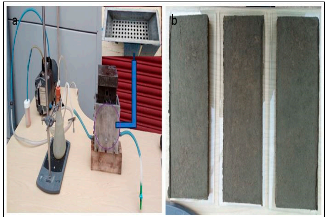
Figure 3. (a) Setup for the lab-simulated Hatschek process. (b) A selection of manufactured specimens in the lab.
