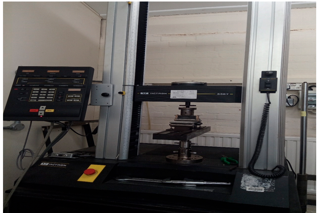
Figure 4. Bending test of specimen in the lab using the Instron 4467 Electromechanical Testing Machine, Norwood USA.
