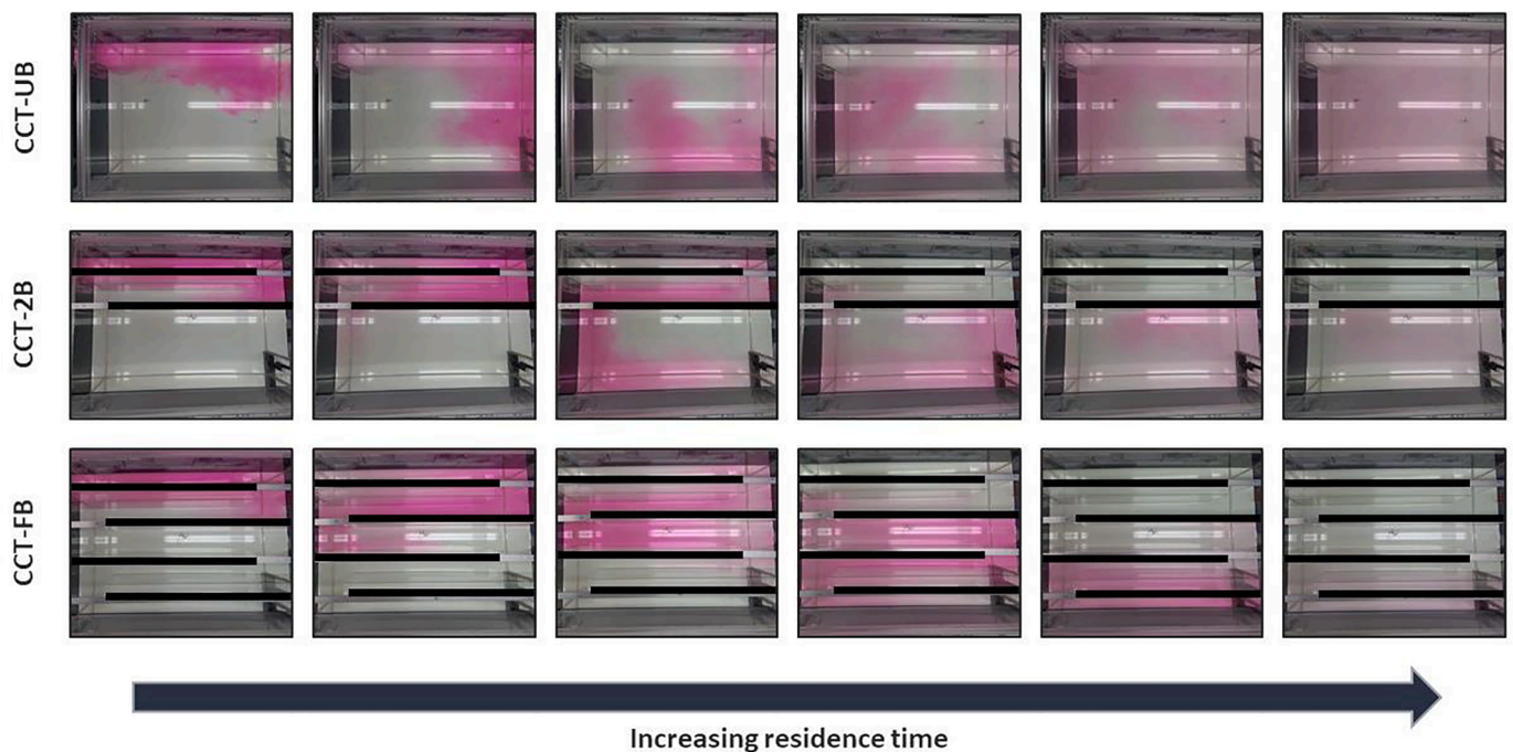
Fig. 3. Images of the rhodamine tracer in the pilot CCT captured over the theoretical residence time. Inlet and outlet locations are indicated by arrows and are in the same location for each test.
