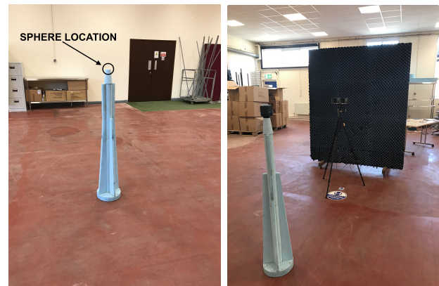
Fig. 1. Experiments setup with the sphere on the styrofoam (left) and with the laser-level system (right).
