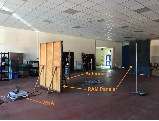
Fig. 2. Photo of the experimental setup with the VNA and the RAM panels.
