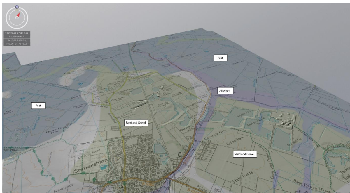
Figure 7: The distribution of sand and gravel extraction in relation to superficial sand and gravel deposits (BGS 1:50 000 [shapefile geospatial data] superficial geology supplied by Edina Geology Digimap Service; Contains Ordnance Survey data © Crown Copyright and database right [2014]).
