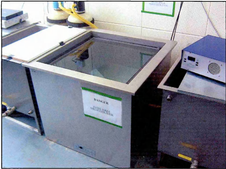
Fig 3.5: Custom built 2kW ultrasound tank.
