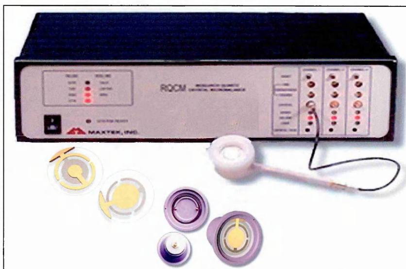
Fig 3.9: RQCM Real-Time Crystal Frequency, Mass and Conductance Measurement Analyser, research crystals and crystal holder.
