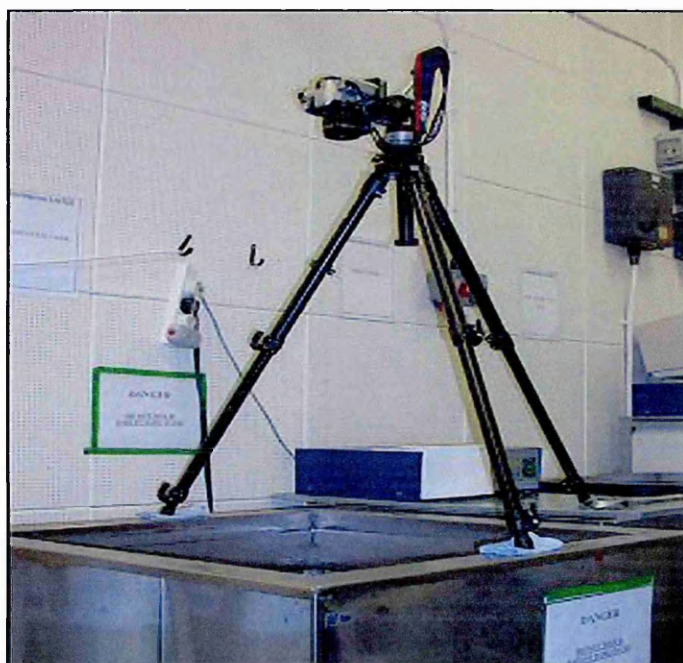
Fig 3.10: Experimental set-up for the photographic recording of sonoluminescence.
