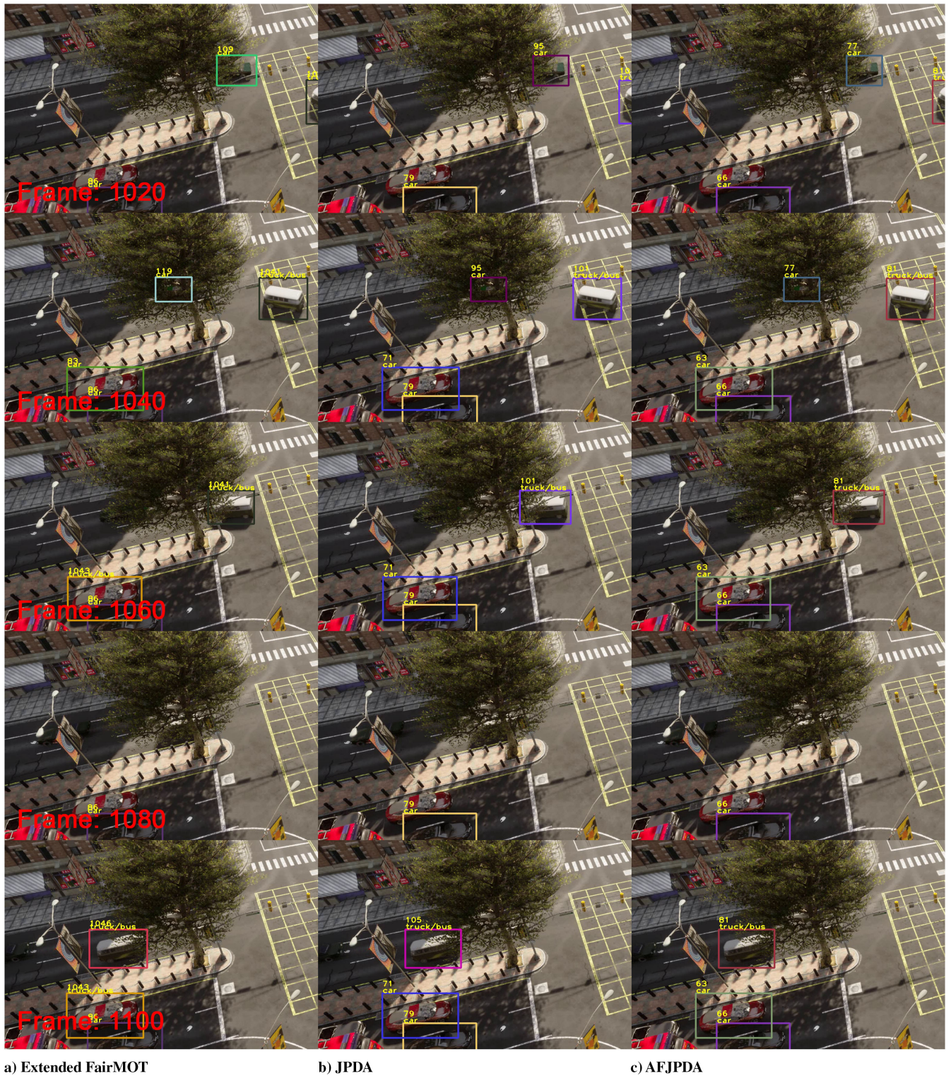
Fig. 7 Tracking results of a) extended FairMOT, b) JPDA filter, and c) AFJPDa filter in the third scenario.
