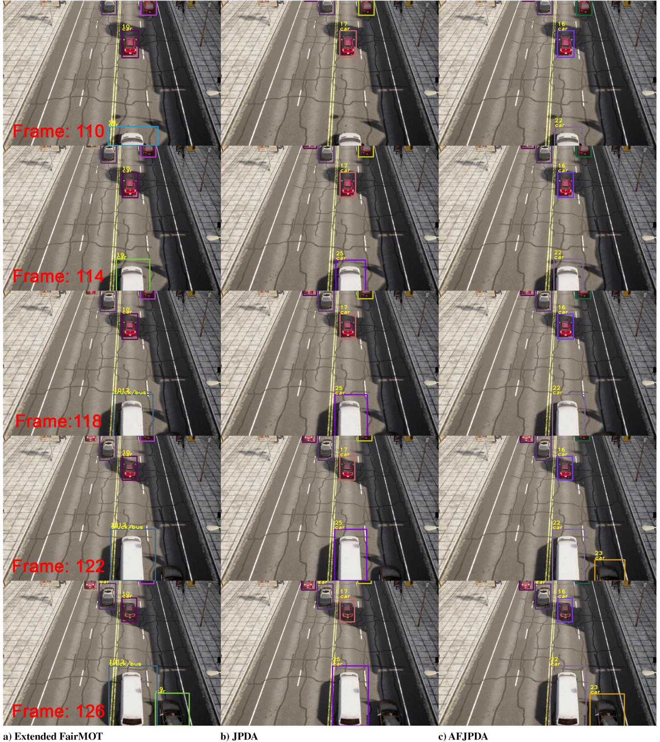
Fig. 6 Tracking results of a) extended FairMOT, b) JPDA filter, and c) AFJPDA filter in the second scenario.
