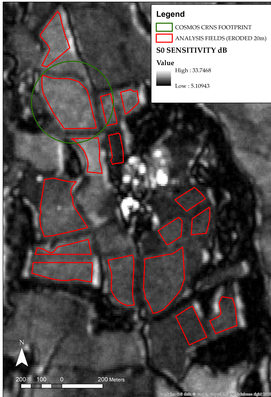
Figure 4.8: Grey-scale image of sensitivity, S calculated for both ascending and descending orbits from 2015-2019 for Sentinel-1 images over the area of North Wyke. The effect of the layover on sensitivity can be seen as bright fringes of abnormally high values of S close to high hedges and the edges of wooded areas. This is particularly noticeable where these boundaries run approximately North/South. Soil moisture estimation in these zones requires special measures to be taken. The eroded field boundaries (in red) appear to exclude most of these areas.
