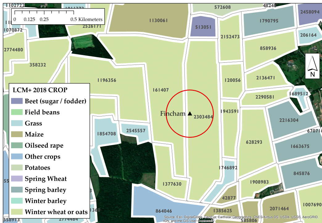
Figure 4.32: Fields surrounding the Fincham site, showing the 200 m footprint (red circle) of the COSMOS-UK CRNS sensor (black triangle). The surrounding fields are labeled by GID, with coloured fill defining the eroded field boundaries used for spatial averaging and the crops that were grown in 2018.
