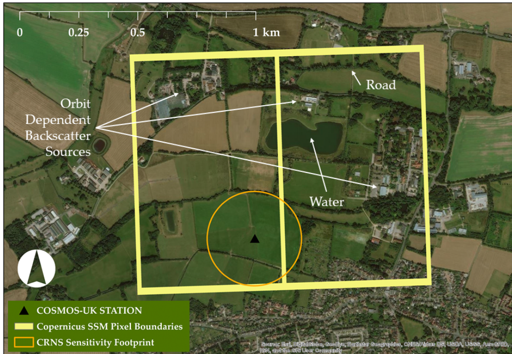
(a) Overlap between Copernicus SSM 1 km pixels and fields at Writtle, showing locations of potential scatter sources. The sensitivity footprint of the COSMOS-UK soil moisture sensor (CRNS) of approximately 200 m radius, is also shown.
