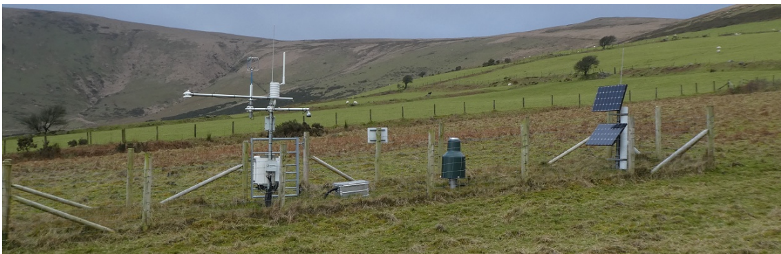
Figure 1.1: Example of a COSMOS-UK soil moisture monitoring station at Cwm Garw, Wales. The Cosmic Ray Neutron Scattering (CRNS) soil moisture sensor is housed in the white tube on the right, vertically mounted, behind the solar panels. Image from COSMOS-UK website ( UK Centre for Ecology and Hydrology, 2021 ).
