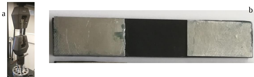
Figure 3. Tensile test + laser strain recording (a)/ Tabs (b)
