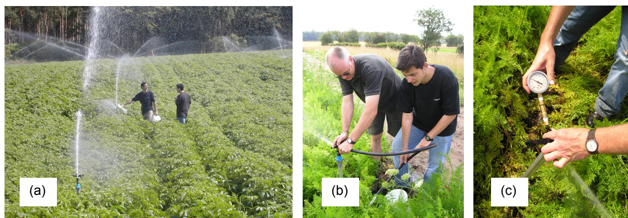
Figure 2.6: Measuring (a) uniformity, (b) discharge and (c) water pressure under sprinkler irrigation in 2005
