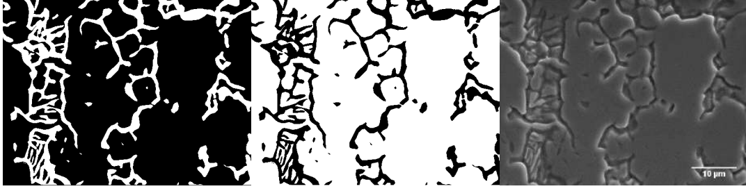
Figure B.3: SEM images after plasma etching and thresholded for (a) only the \alpha phase, (b) only the \beta phase and (c) original SEM image for position C in Figure 4.13
