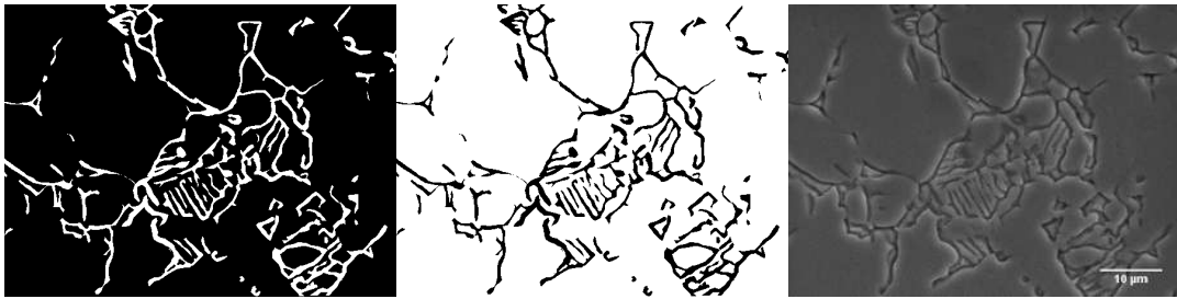
Figure B.5: SEM images after plasma etching and thresholded for (a) only the \alpha phase, (b) only the \beta phase and (c) original SEM image for position E in Figure 4.13
