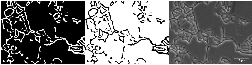
Figure B.1: SEM images after plasma etching and thresholded for (a) only the \alpha phase, (b) only the \beta phase and (c) original SEM image for position A in Figure 4.13
