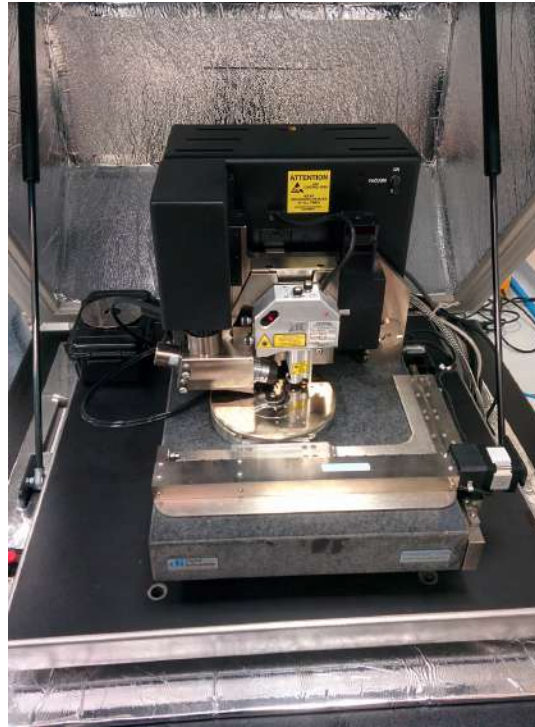
Figure 3.15: Bruker Veeco Dimension 3100 AFM machine.
