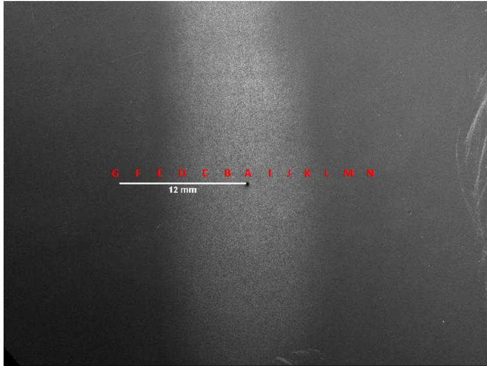
Figure 4.13: Wide field SEM image at 6x magnification of Ti64 surface after plasma etching and polishing. The trench is etched at a processing speed of 100 \text{ mm min}^{-1} .
