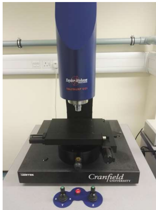
Figure 3.13: Talysurf 6000 coherence correlating interferometer (CCI) setup.
