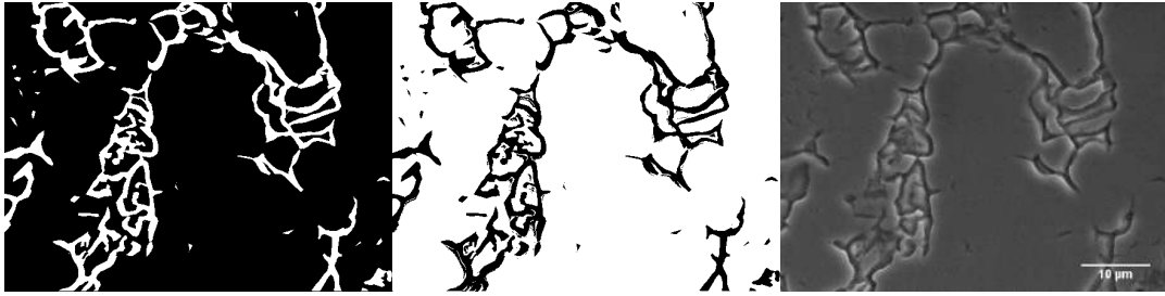
Figure B.4: SEM images after plasma etching and thresholded for (a) only the \alpha phase, (b) only the \beta phase and (c) original SEM image for position D in Figure 4.13
