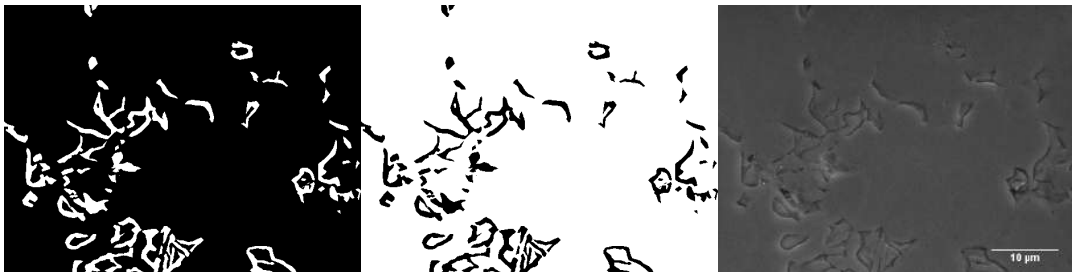
Figure B.6: SEM images after plasma etching and thresholded for (a) only the \alpha phase, (b) only the \beta phase and (c) original SEM image for position F in Figure 4.13
