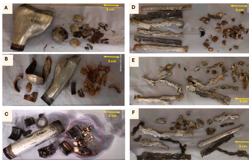
Fig. 3. Pipe bomb fragments produced from low order detonations (A-B), partial detonation (C) the red circle shows the undetonated TNT and high order detonations (D-F).
