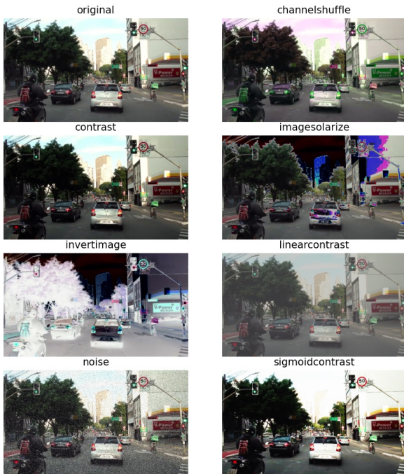
Figure 4. Example of the augmentation methods on one image from the dataset. Source: [Pierre and Fernandes, 2023].
