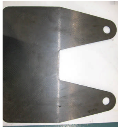
Figure 7. 12 layer NCF preform before hole cutting Figure 8. RTM moulding after edge deflashing
