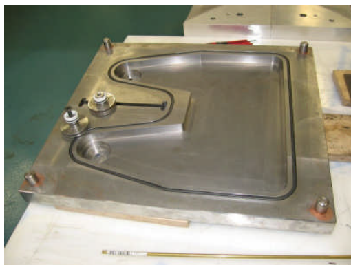
Figure 6. RTM mould tool base with hole inserts
