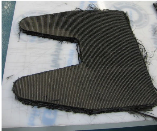
Figure 7. 12 layer NCF preform before hole cutting Figure 8. RTM moulding after edge deflashing
