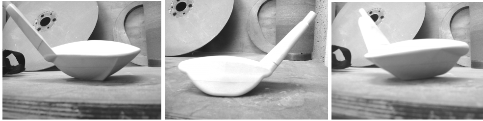
Figure 64: final pictures of the golf club numerically computer controlled cut
