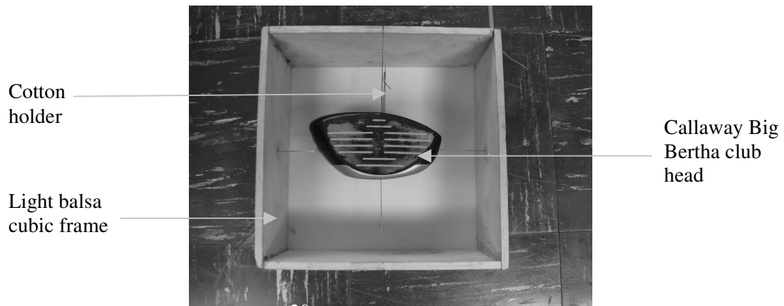
Figure 12: Callaway Big Bertha Club head in balsa frames (the cottons represent the two orthogonal axes)
