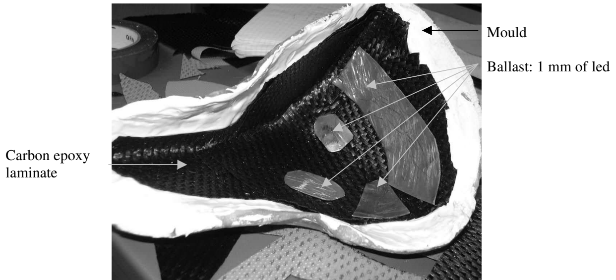
Figure 71: the ballast in the prototype
