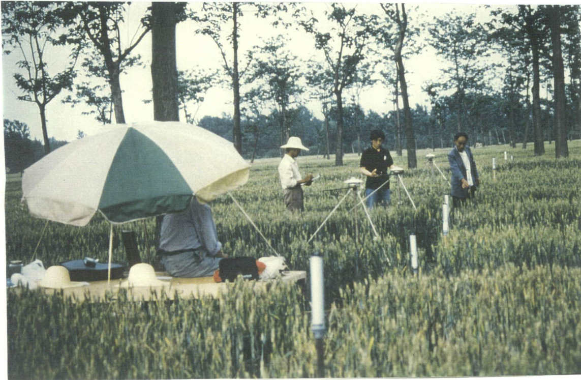
Plate 4.3. Automatic Radiation Station in use along a transect with Digital PAR integrator (right hand side) in 5x30 m paulownia-wheat intercropping field at Dangshan, Anhui Province, China 1993.
