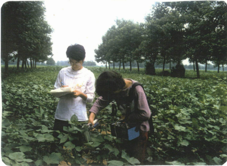
Plate 4.5 LI - 1600 stable porometer used in paulownia - cotton field which was also used in measuring the physiological variables of winter wheat and other summer crops.
