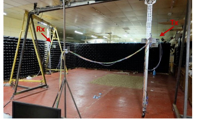
Fig. 1. The GBSAR laboratory in a bistatic configuration.
