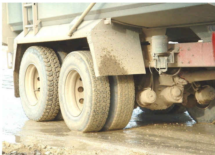
Figure 8 tyre and chassis contamination resulting from driving on unsurfaced roads within a quarry
