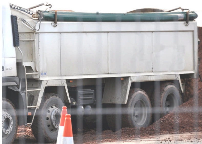
Figure 37 – Lateral sheet system fitted to an insulated tipper body.
