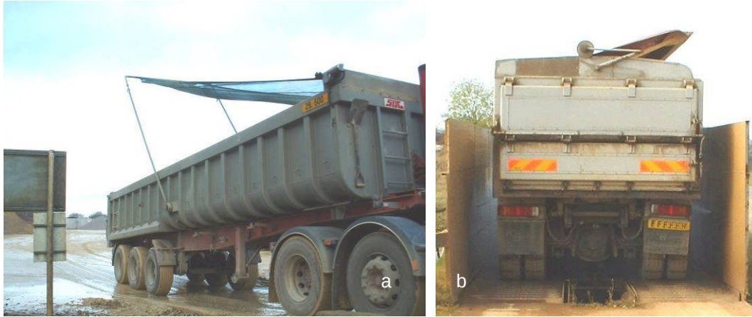
Figure 12 Longitudinal (a) and lateral (b) load covers used on aggregate trucks
