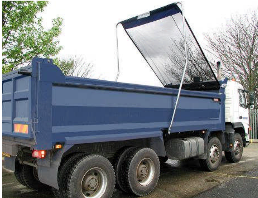
Figure 36 – Longitudinal sheet system
