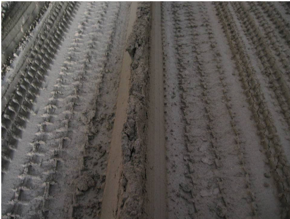
Figure 29 – Soil surface after 10 passes.
