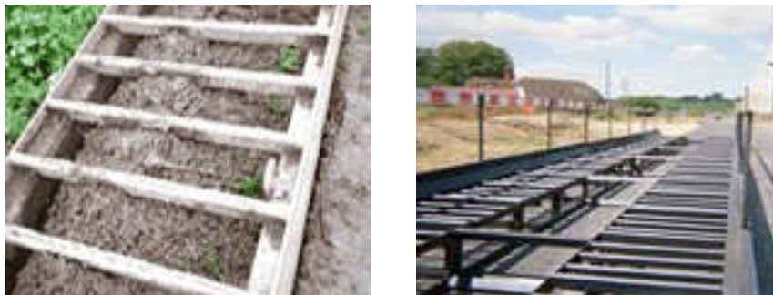
Figure 10 A vibrating grid type tyre cleaner (Econoclean Systems Ltd.)
