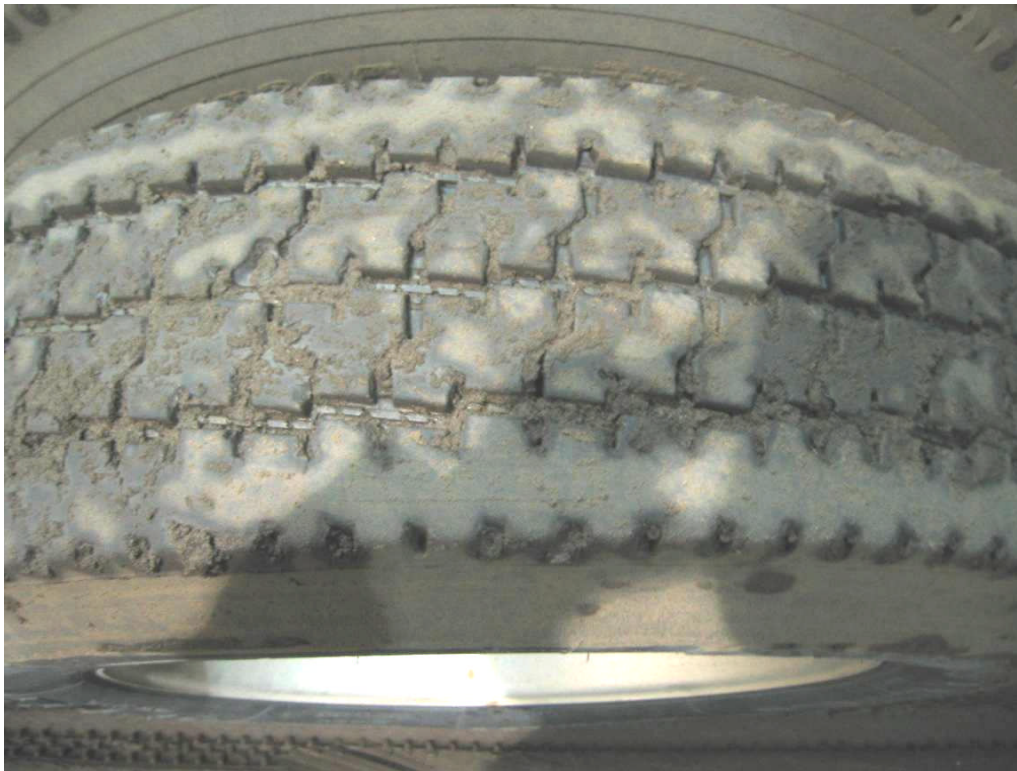
Figure 30 – Typical tyre condition after 10 passes.
