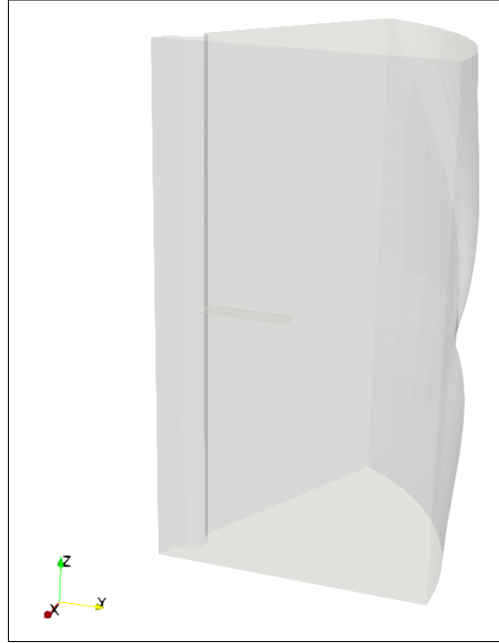
Figure 4.8: Figure depicts the quarter domain of the Application to rotating wings (Caradonna and Tung rotor) case.
