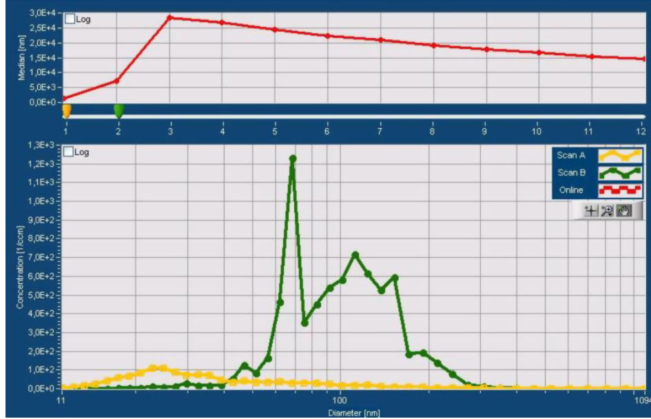
Figure 3.19: SMPS on-line measurement of the particle size distribution (difference in the natural logarithm of the particle concentration vs. mean particle size) during drilling; the green line represents the actual measurement and the yellow line represent the previous measurements
