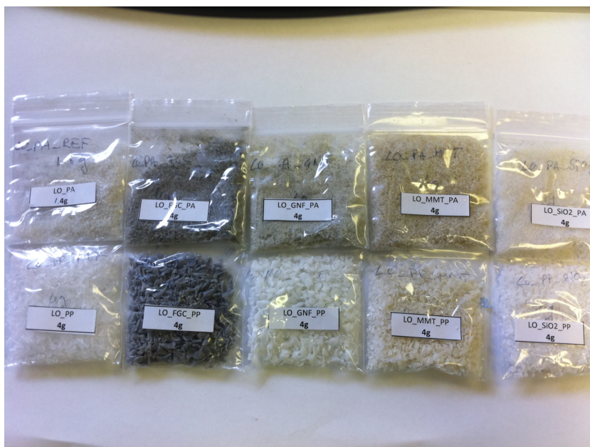
Figure 3.25: Set of dry particles sampled from drilling of nanocomposites
