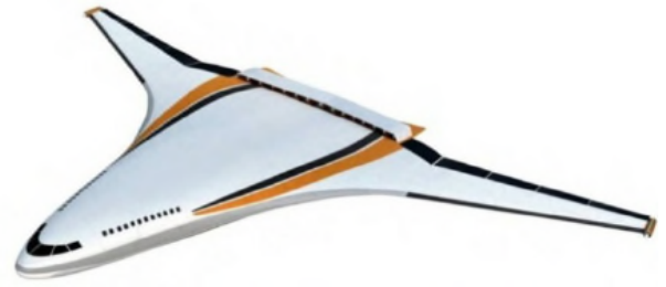
Figure 6 TeDP on a blended wing body airframe [47]
