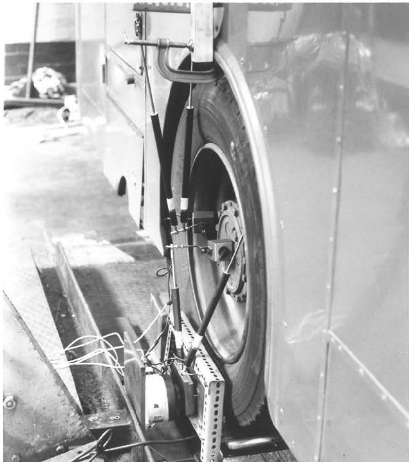
Figure 3.13 Force and Displacement Transducers for Tilt Test
