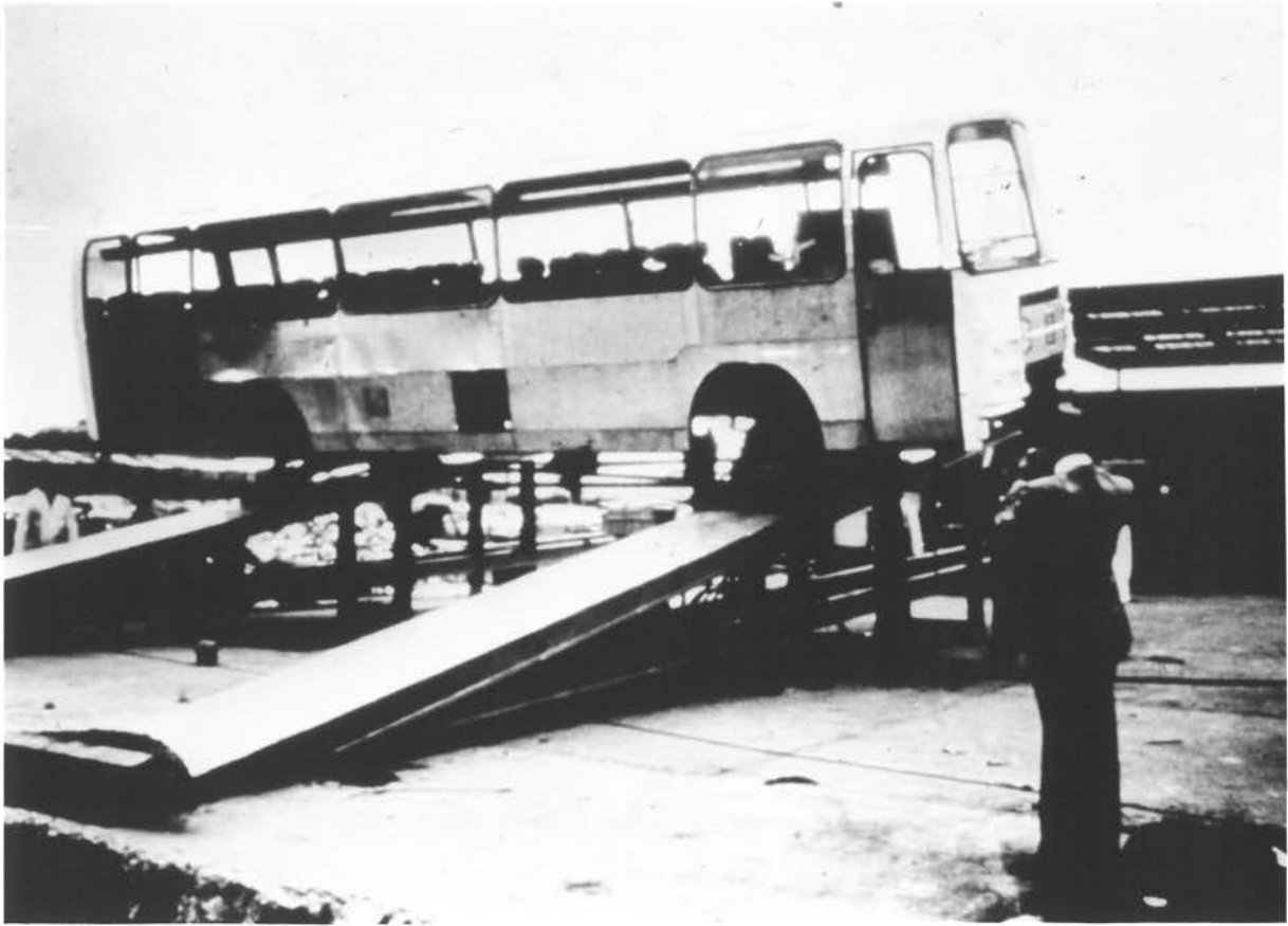
Figure 2.1 Before Superstructure Strength Test
