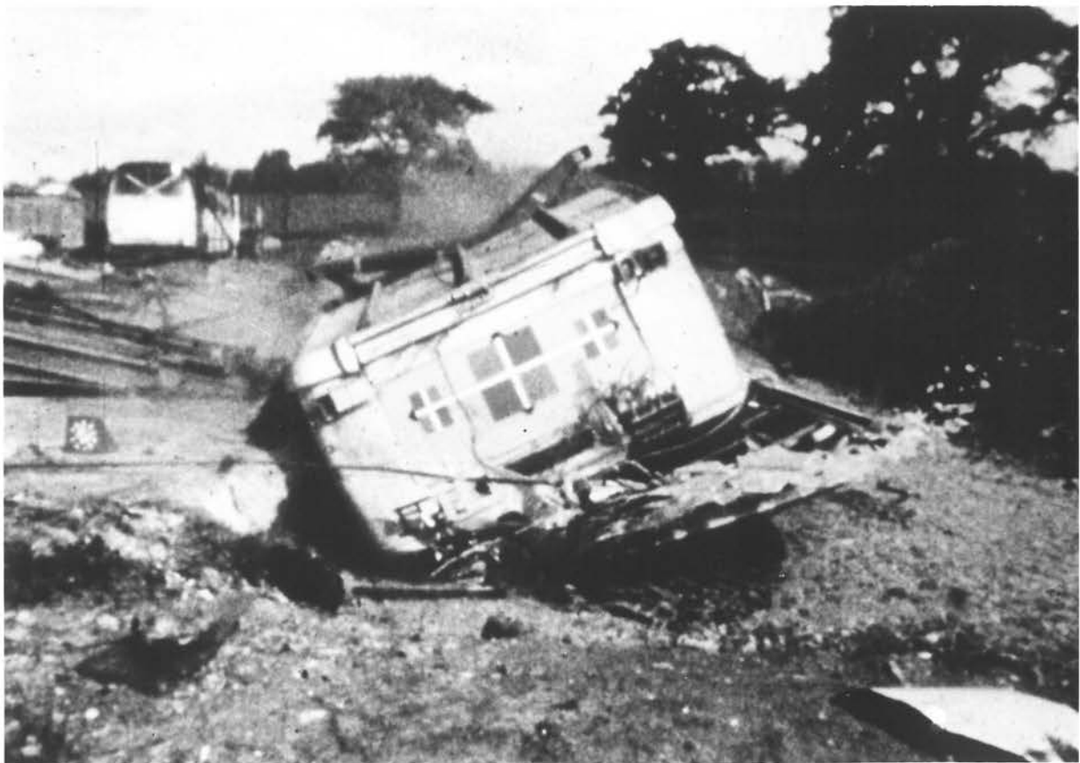
Figure 2.2 After Superstructure Strength Test
