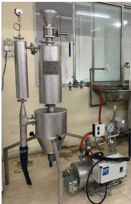
Thermal Hydrolysis Reactor TS = 14.0%
