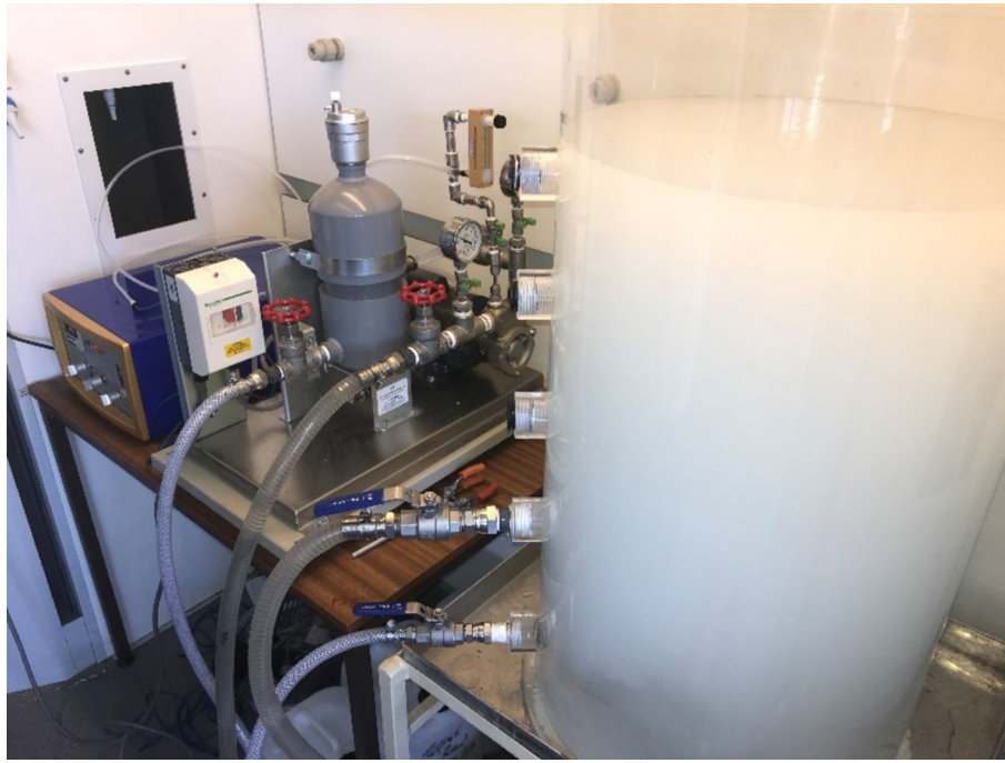
Fig. 1. Microbubble generation experimental apparatus.
