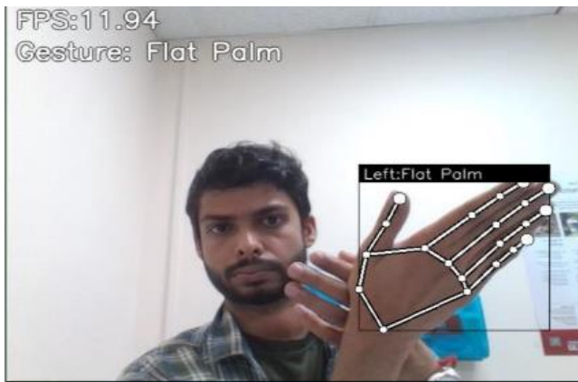
Figure 4: Both hands are not detected as one hand is occluded by other hand.
