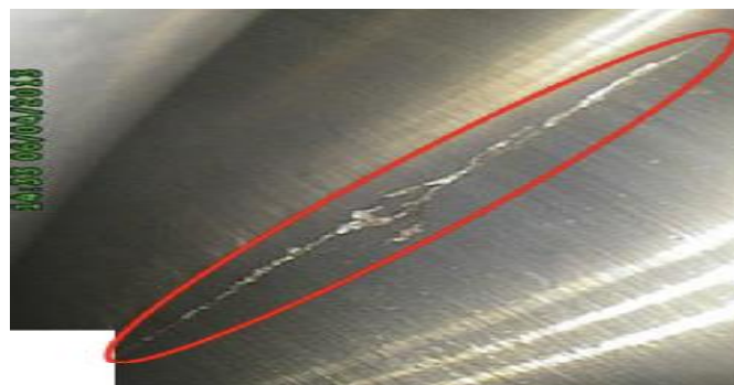
Figure 2: Wind turbine high-speed shaft bearing defect (Bechhoefer et al. 2013)
