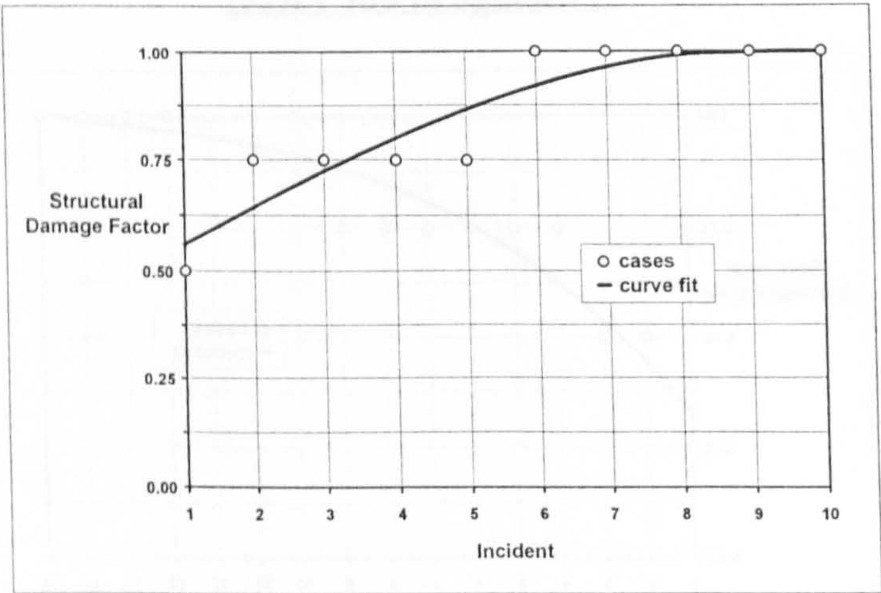
Figure C.5: Fuselage Structural Damage Levels (Fuselage in Three Pieces: Centre Section)
