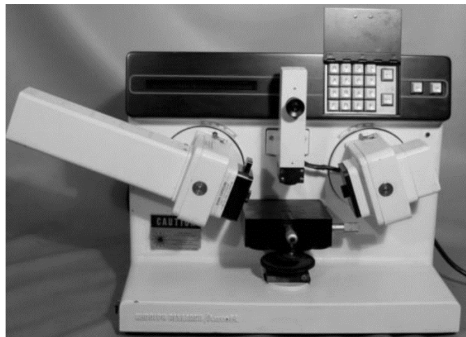
Figure 15: Rudolph Ellipsometer AutoEL used in the experiments.
