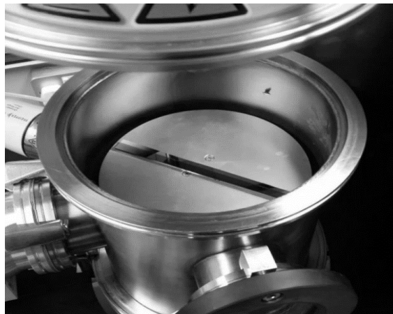
Figure 21: Silicon strip taped down across the rotary table using Kapton tape.
