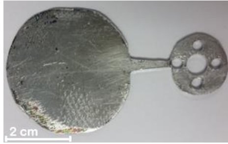
Figure 32: Mask #1 made of 1 mm thick aluminium.
