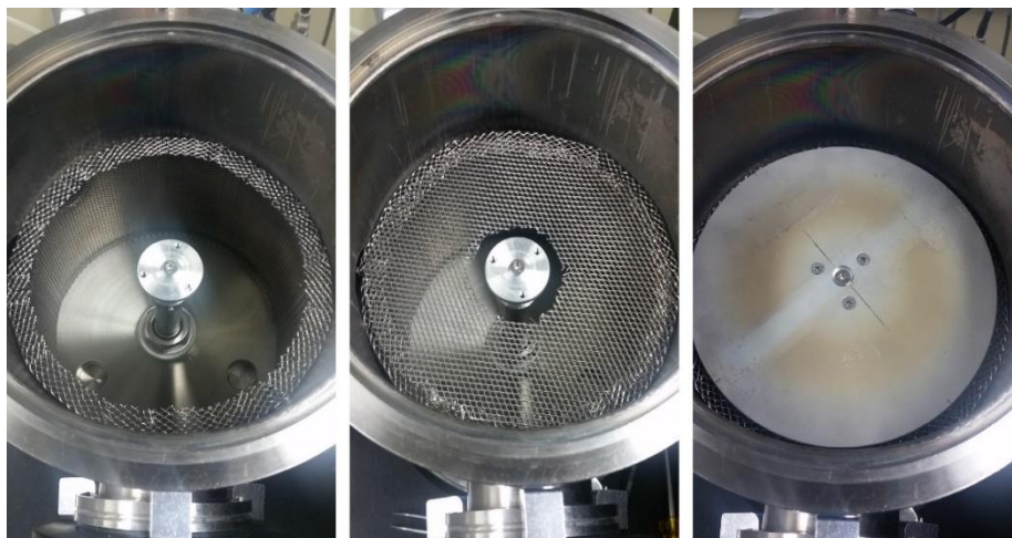
Figure 57: Mesh installation in the chamber.
